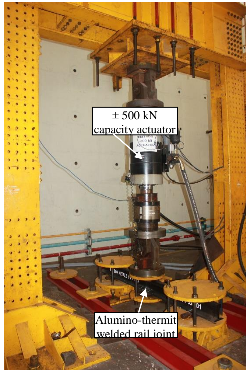
Set-up for fatigue test on an alumino-thermit welded rail joint
