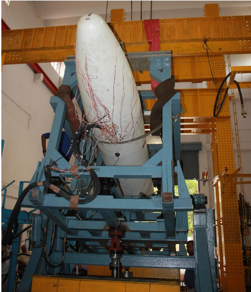
Fig. 1 Typical views of fuel drop tank during simultaneous slosh and vibration test
