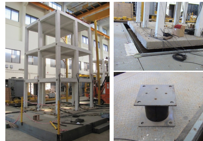
Shake table testing of RCC frame with seismic base isolation devices
