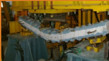
LSCC system for blast resistance
