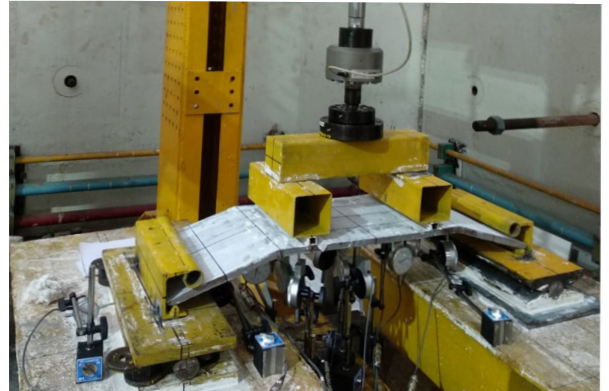
Flexure test on folded TRC fence panels
