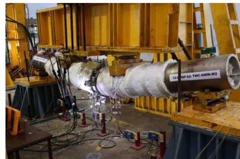
Deflected shape of the dissimilar pipe weld joint after fracture test at elevated temperature
