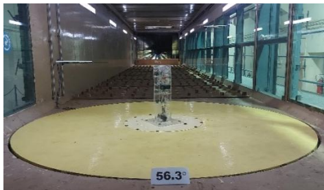
Wind tunnel testing of 1:1.5:6 rectangular building model
