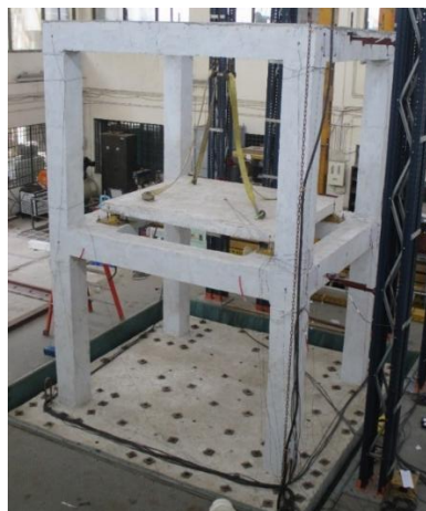
Shake table testing of building frame with floor mass isolation
