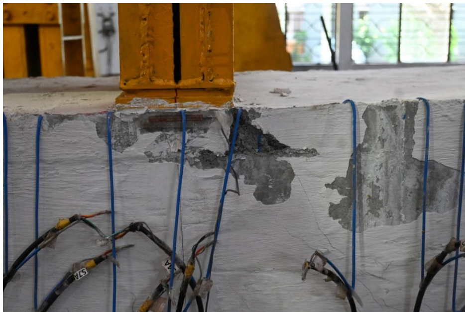
Failure of the specimen by concrete crushing at top compressive fiber
