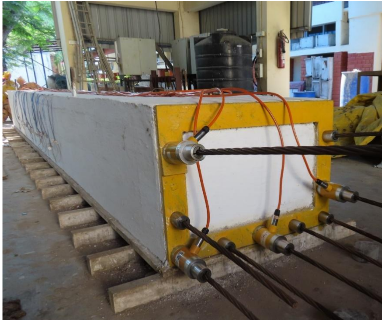
Specimen CBG3-SM after completion of post-tensioning. Monitoring of prestress using Vibrating Wire Load cells is shown.
