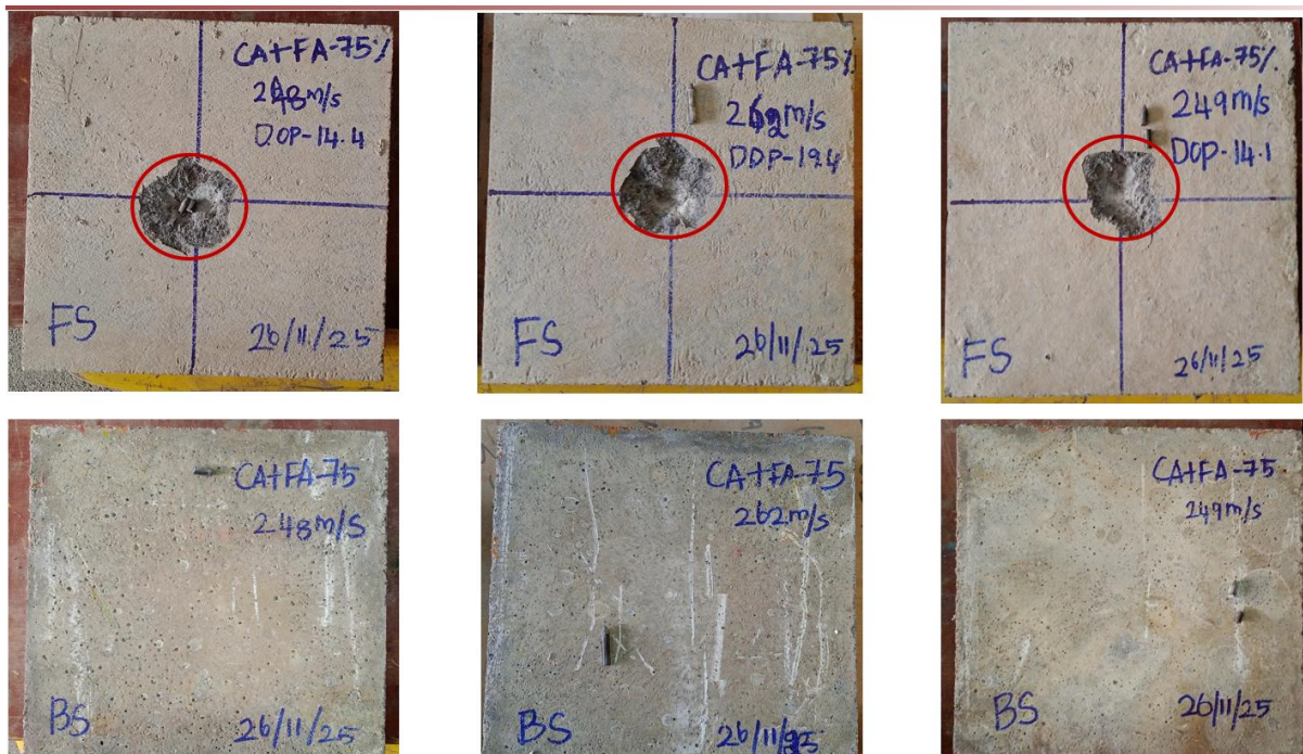
Damaged panels under ballistic impact
