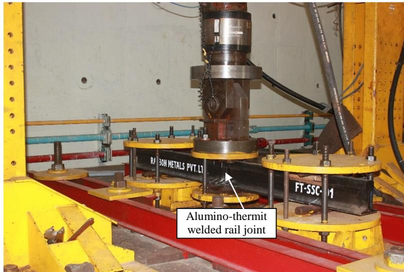
*Close-up view of the test set-up*
