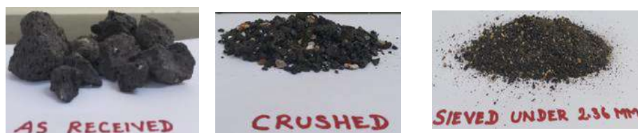
Fig. 1 a) As received b) Crushed in jaw crusher c) Crushed aggregate passed in 2.36 mm sieve
