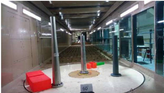
Fig. 1 View of the models of chimneys with interfering bodies in wind tunnel for typical angles of wind incidence (60° and 330°)
