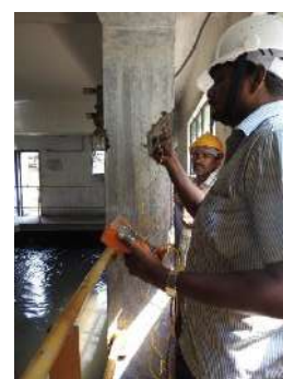
Fig. 2 Half-cell potential measurements on a typical column
