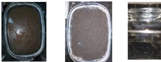
Fig. 2. Water absorption test a) Slag aggregate immersed in water b) Slag aggregate in saturated surface dry condition c) Aggregate in oven
