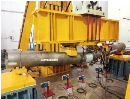
Deflected shape of the pipe weld joint after fracture test
