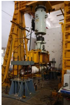
Set-up for cyclic fracture test under cyclic loading
