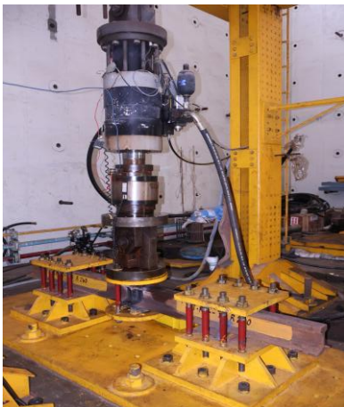
Set-up for fatigue test on alumino-thermit welded rail joint
