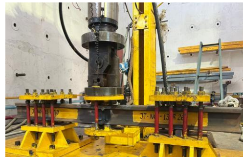
Close-up view of fatigue test set-up
