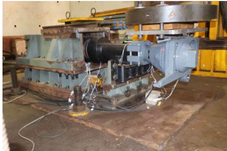
Set-up for vertical shear strength test on coupler head with draft gear
