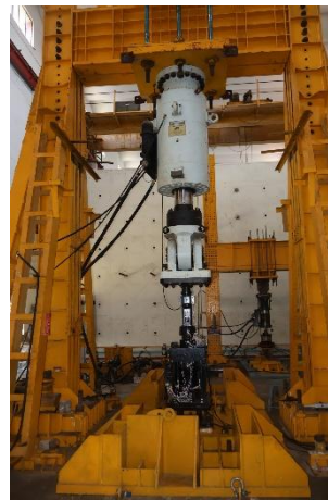
Set-up for endurance test on draft gear
