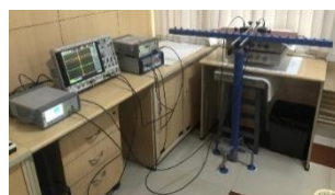
Air-coupled (noncontact) ultrasonic testing set-up
