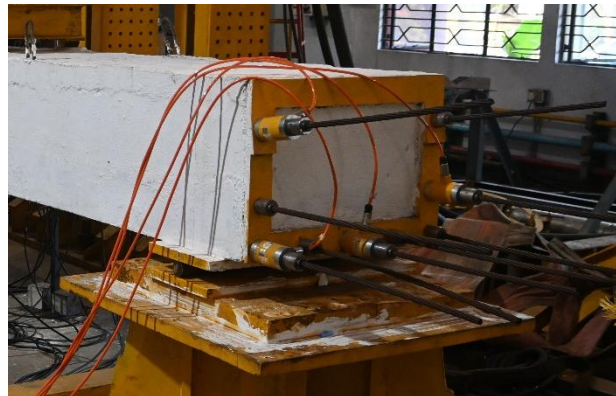
Monitoring the prestress using vibrating wire load cells
