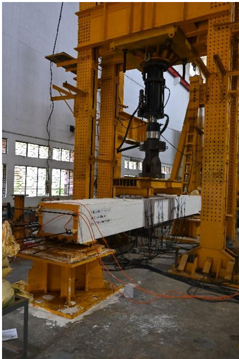
Testing of the PSC box girder specimen CBG2-SM subjected to static monotonic load
