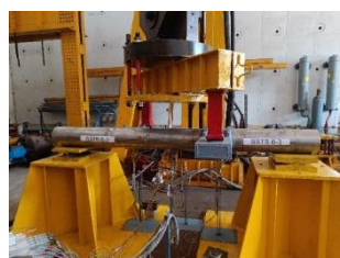
FCG test on a straight pipe under combined bending and torsion
