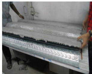
Production of TRC roofing sheet using TRCPT
