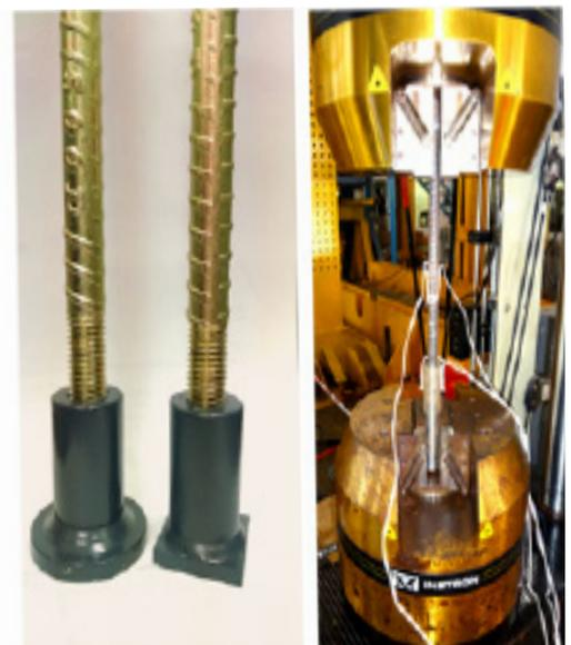
Head-T rebar end anchors
