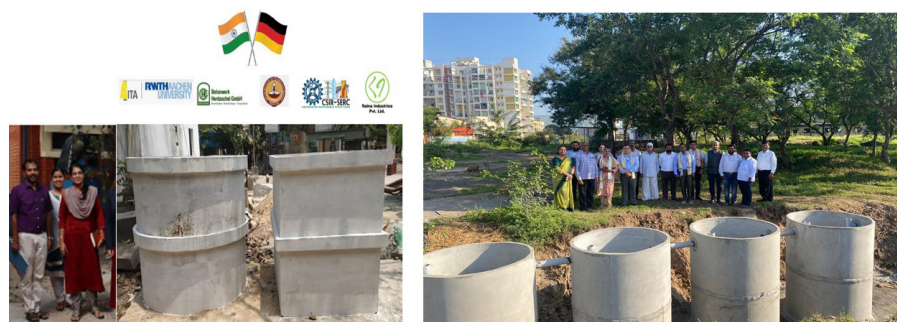
Modular lightweight wastewater treatment units made with TRC for rural and periurban dwellings (CleanWater)
