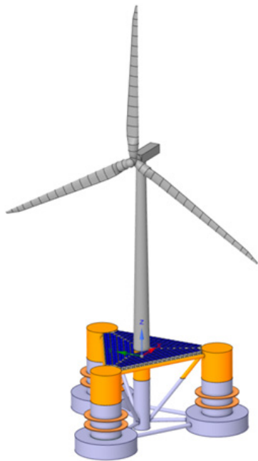
Fig. 6 Free decay experiments on semisubmersible platform with hybrid offshore wind turbine and solar farm
