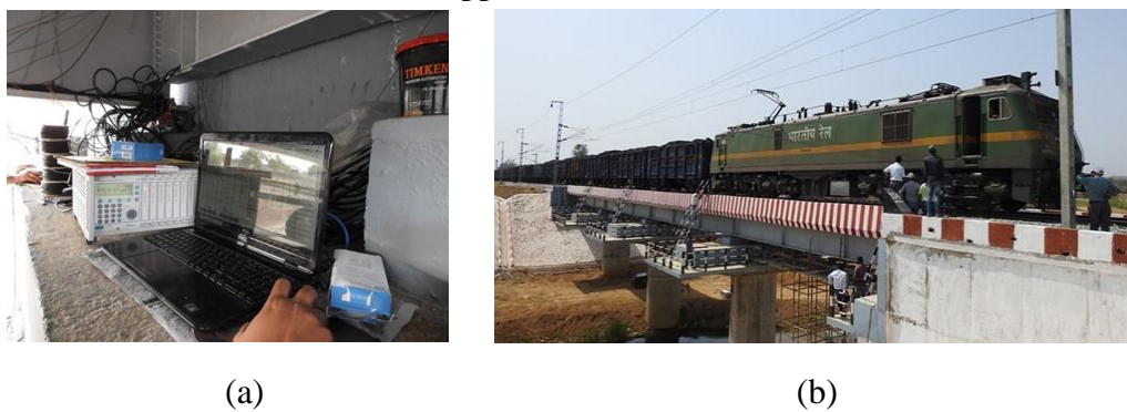
Fig. 3: (a) High accuracy data acquisition system and (b) test train formation for loading
