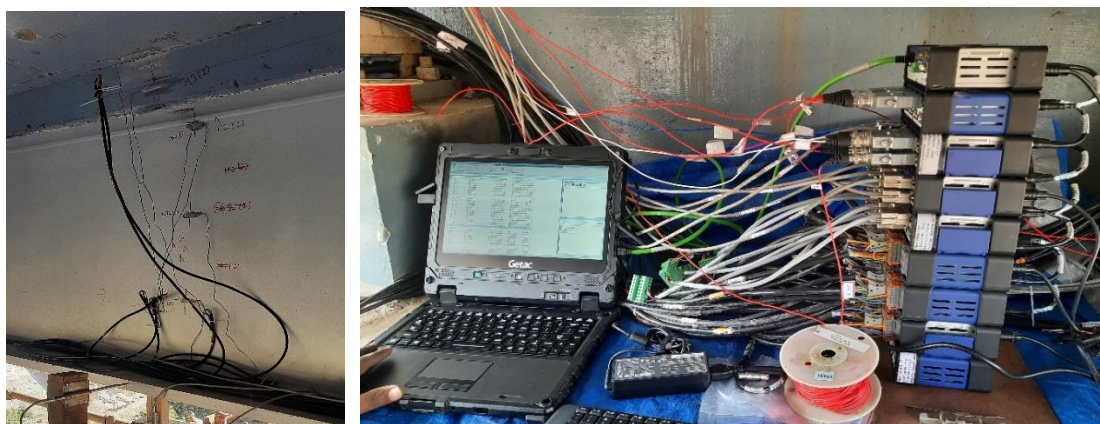
Figure Sensors in steel-concrete composite and Instrumentation
