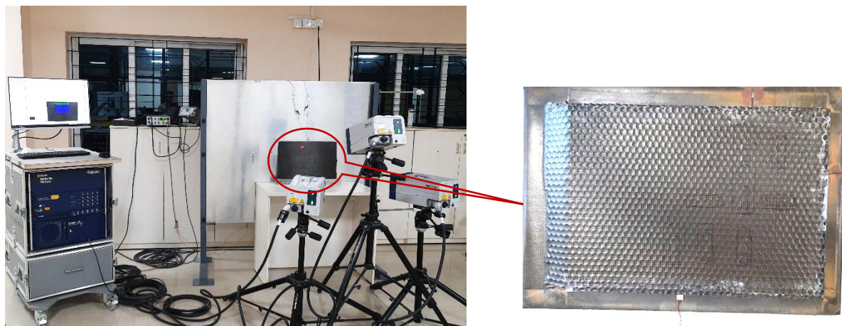
Fig. 1: (a) Experimental setup and (b) Linear composite honeycomb panel
