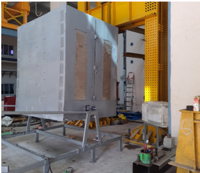
Vertical Mode: for testing of column members
