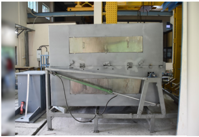
Horizontal Mode: for testing of beam members
