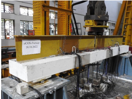
Experimental test set-up for investigations (inverted position)
