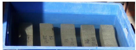
Typical water absorption test
