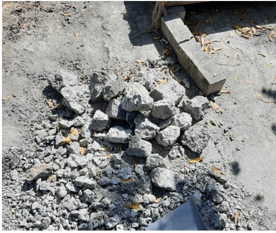
Typical recycled concrete aggregate
